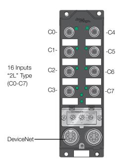
This busstop® station takes in up to sixteen discrete three-wire inputs or eight discrete four-wire input points per node. There are two inputs per connectorone on pin four and one on pin two. Each input automatically detects a sourcing (PNP) or sinking (NPN) open-collector signal. Any combination of NPN and PNP devices may be used.
